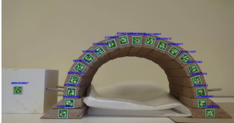
Figure 4.12: 3D-scaled model of the arch and the tracked markers by DeepTag
