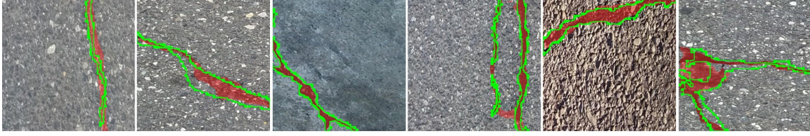
Figure 3.1: Six samples of crack detection and segmentation. The red area has predicted by our model and the green line is the ground truth border.
